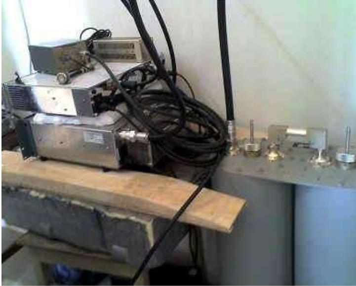
**Figure 9 - Testing the transmitter and filter**
