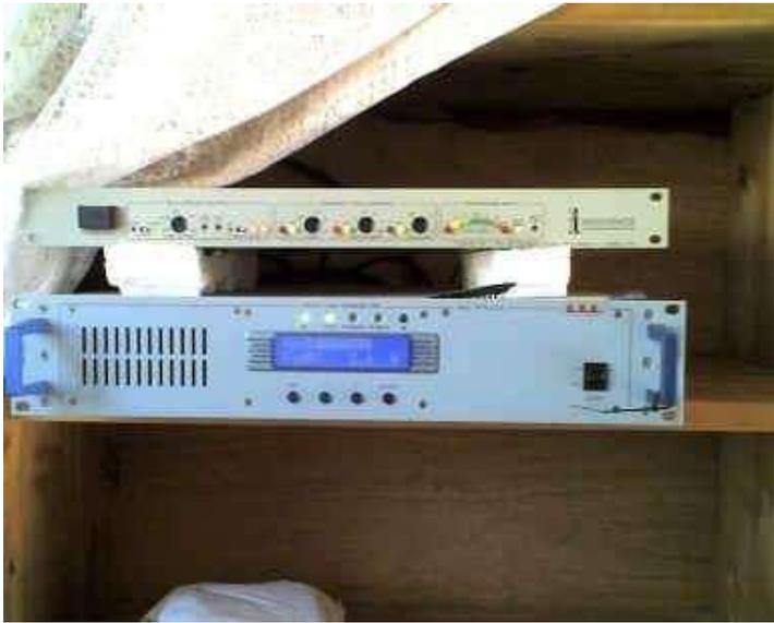
**Figure 5 - Audio processor/encoder and Studio-to-Transmitter Link (STL) transmitter at the studio**
