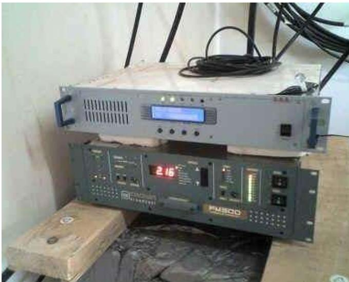
**Figure 6 - STL Receiver and 300-watt transmitter on Mafifi Hill**
